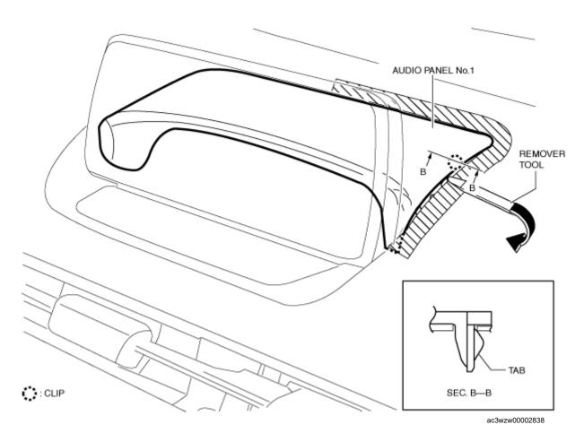
5. Insert the remover tool into the position shown in the figure.
