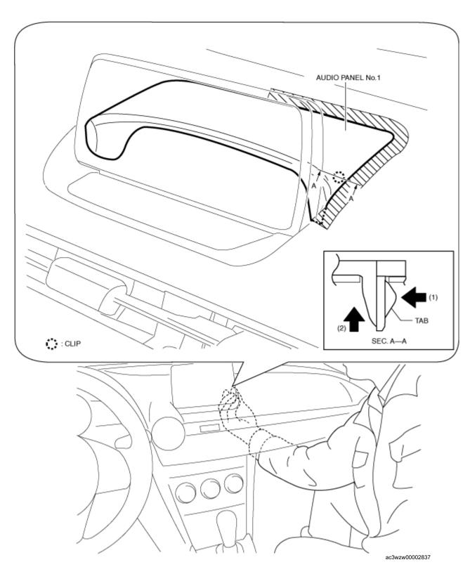
4. Insert the remover tool into the clearance assured in Step 3, move the remover tool in the direction of the arrow shown in the figure and lift up the audio panel No.1.
