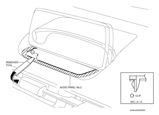
5. Remove audio panel No.2 by pulling it in the direction of the arrow shown in the figure.
