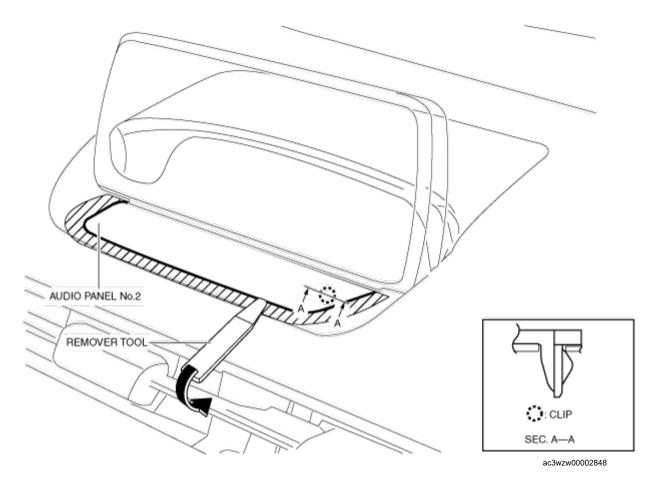
3. Insert the remover tool into the position shown in the figure, move the tool in the direction of the arrow and detach the clip from the dashboard.
