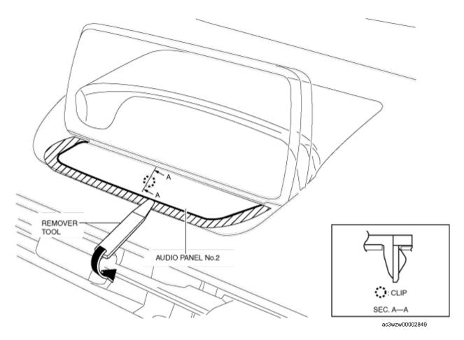
4. Insert the remover tool into the position shown in the figure, move the tool in the direction of the arrow and detach the clip from the dashboard.
