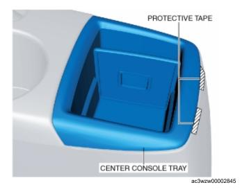
2. Insert a remover tool into the positions shown in the figure, move it in the directions of arrows (1), and detach clips A from the rear console.
