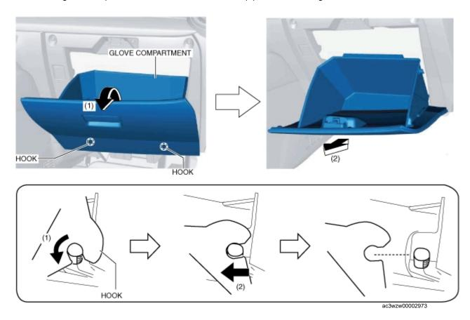
4. Move the glove compartment in the direction of arrow (2) shown in the figure and remove it while detaching the hooks.
